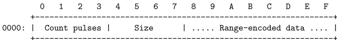
Count pulses: Count of the NRZI transition flux pulses in half track
